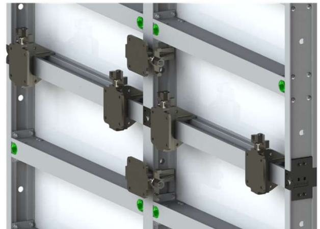
Figure 3. Use Standard Clamps At All Vertical Or Horizontal Panel Joints
